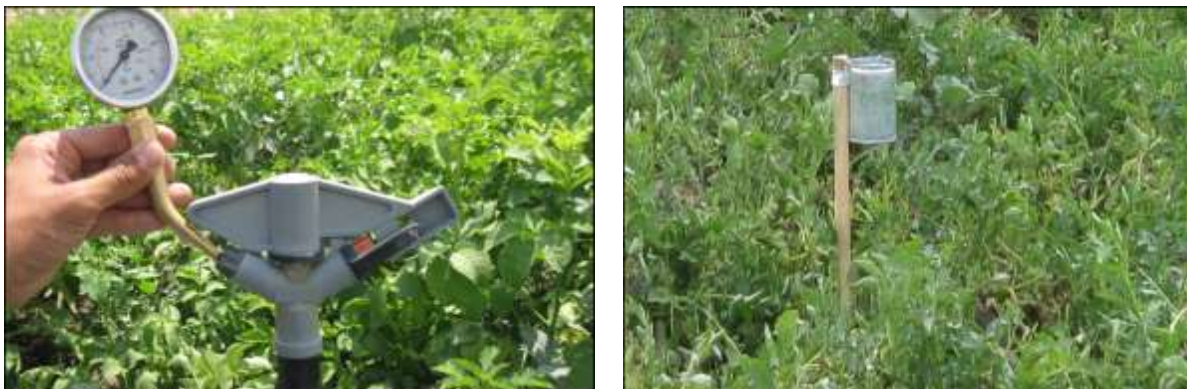
Figure 1. Measuring sprinkler pressure and catch can
