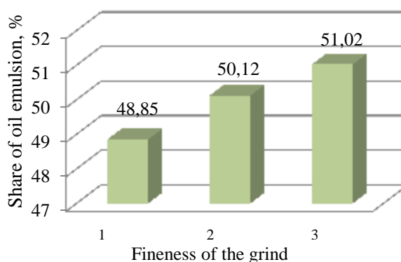
Figure 1 – Fat-emulsifying ability of the amaranth flour with the different fineness of the grind: 1 – 1.0 mm and less; 2 – 0.315 mm and less; 3 – 0.125 mm and less
