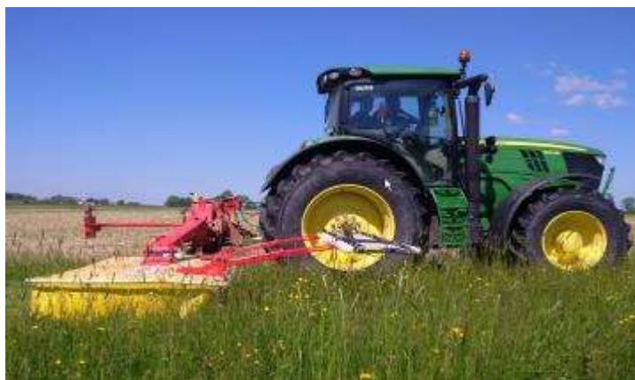
Fig. 3 – Tractor and mower, with sensor bar attached in front of the mower
