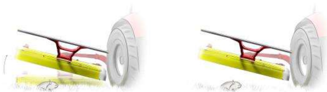
Fig. 4 – a) Mower with knife during and b) after the lifting process
